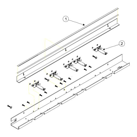
Figure 6-4. C-Bracket Assembly Breakdown.
